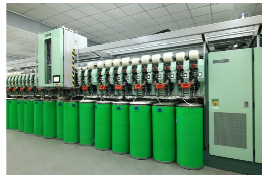
Fig. 1: The air-jet spinning machine J 70 enables the production of high-quality yarns with maximum efficiency. PP-ID: 98480
