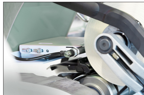
Fig. 2: Smartjet installed in doffer unit to improve the efficiency of the upper yarn search Asset ID: 96425
