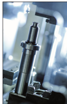
Fig. 2: NASA HPS 68 on production line - the first spindle running at 30.000 rpm PP-ID 36546
