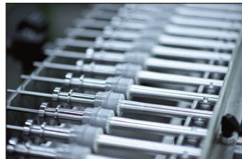
Fig. 3: Spindle top part with the industry proven SERVOGrip, saving yarns and maintenance costs. PP-ID 36533
